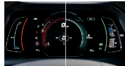
7" LCD instrument cluster (Sport/Normal modes)
