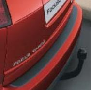
For extra transport and stowage capability, the tow bar can tow up to 1,500 kg depending on engine. Available as fixed and detachable versions. (Option and accessory)
