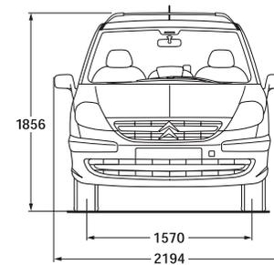
All measurements are in millimetres.
