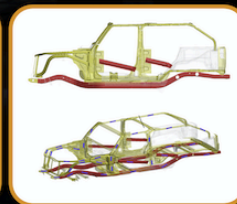
COLLISION SAFETY USING HIGH STRENGTH CARRIER FRAME
