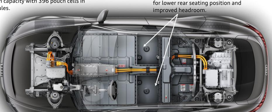
Battery position provides almost perfect 50:50 weight distribution and very low centre of gravity for improved handling.
